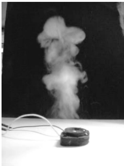
Fig. 5 Image of the piezoceramic disk used in the present experiments, during the atomization process
